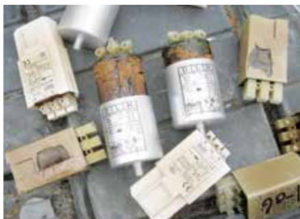
Harmonic distortion of the mains voltage leads to a significantly reduced service life of capacitors.
